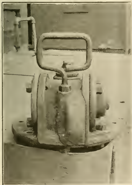
FIG. 2. JIG FOR HANDLING AIR PUMP HEADS IN TRANSIT.
